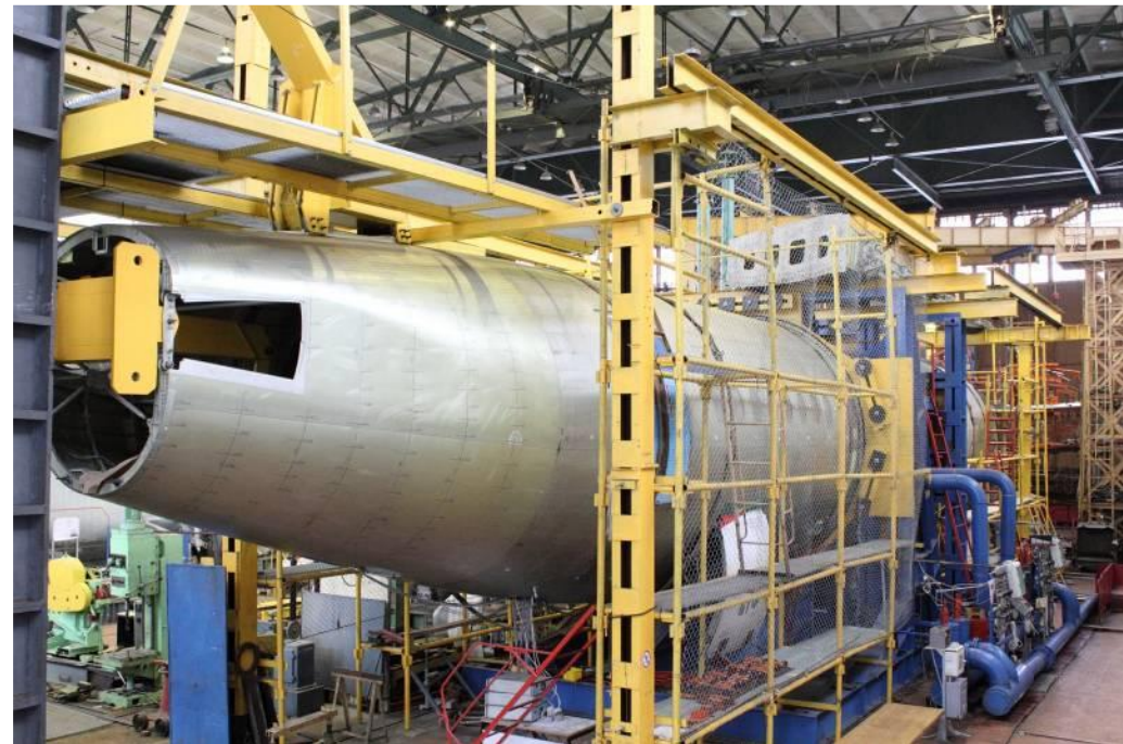
Fatigue tests of the rear compartment of the SSJ- 100 aircraft fuselage
