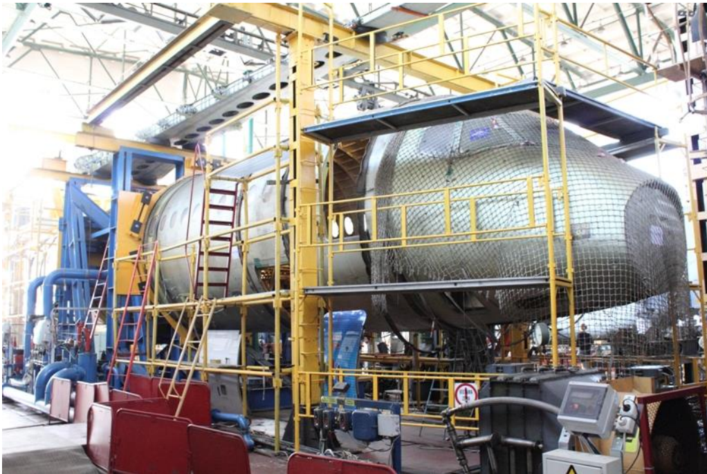
Fatigue tests of the front compartment of the SSJ-100 aircraft fuselage
